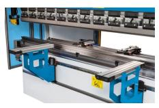
The rigid front support arms feature a ratchet mechanism for quick height adjustments
