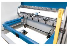
Option: Back gauge with controlled R axis
