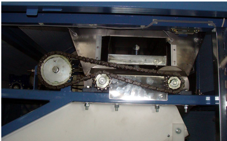
Fig.: Properly connected drive of the segment cylinders
