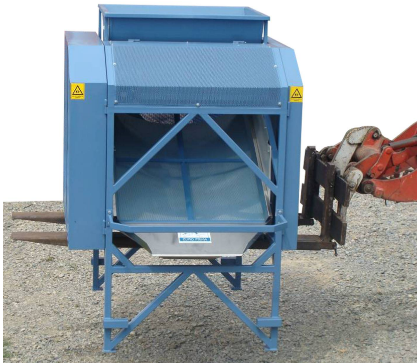
Fig.: Correct lifting of the machine with a forklift
