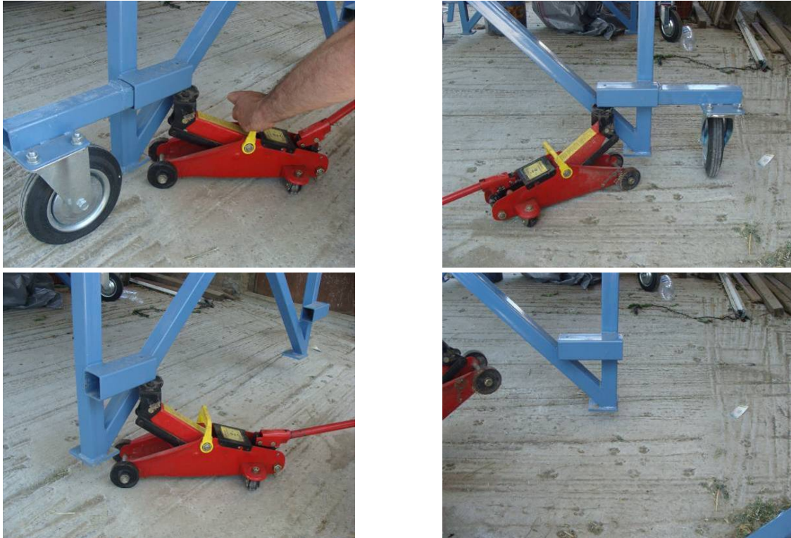
Fig.: Removing the wheels from the machine
