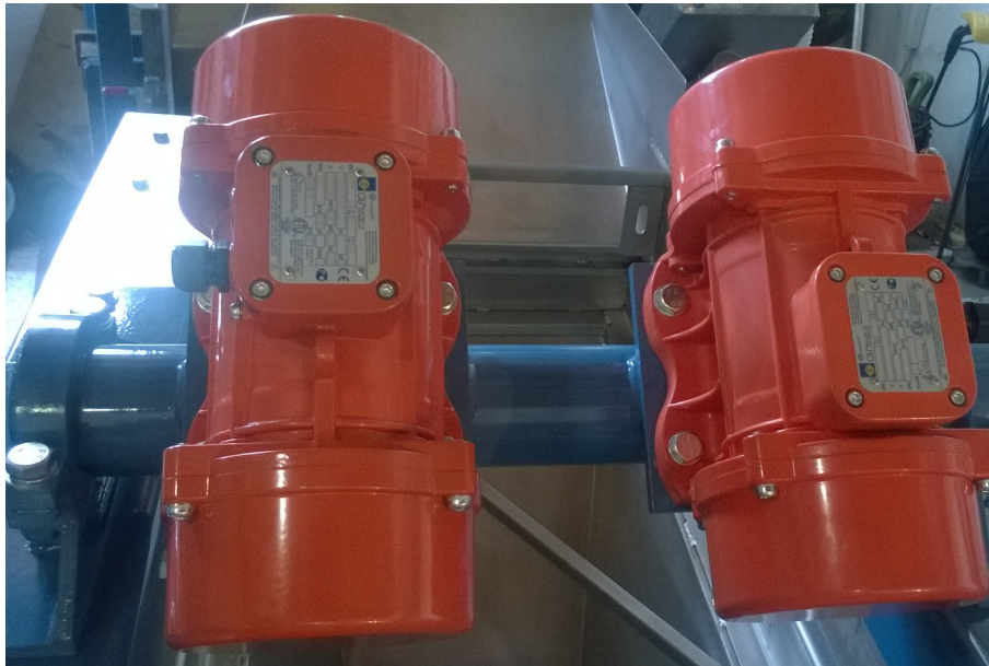
Fig.: Setting the direction of oscillation
