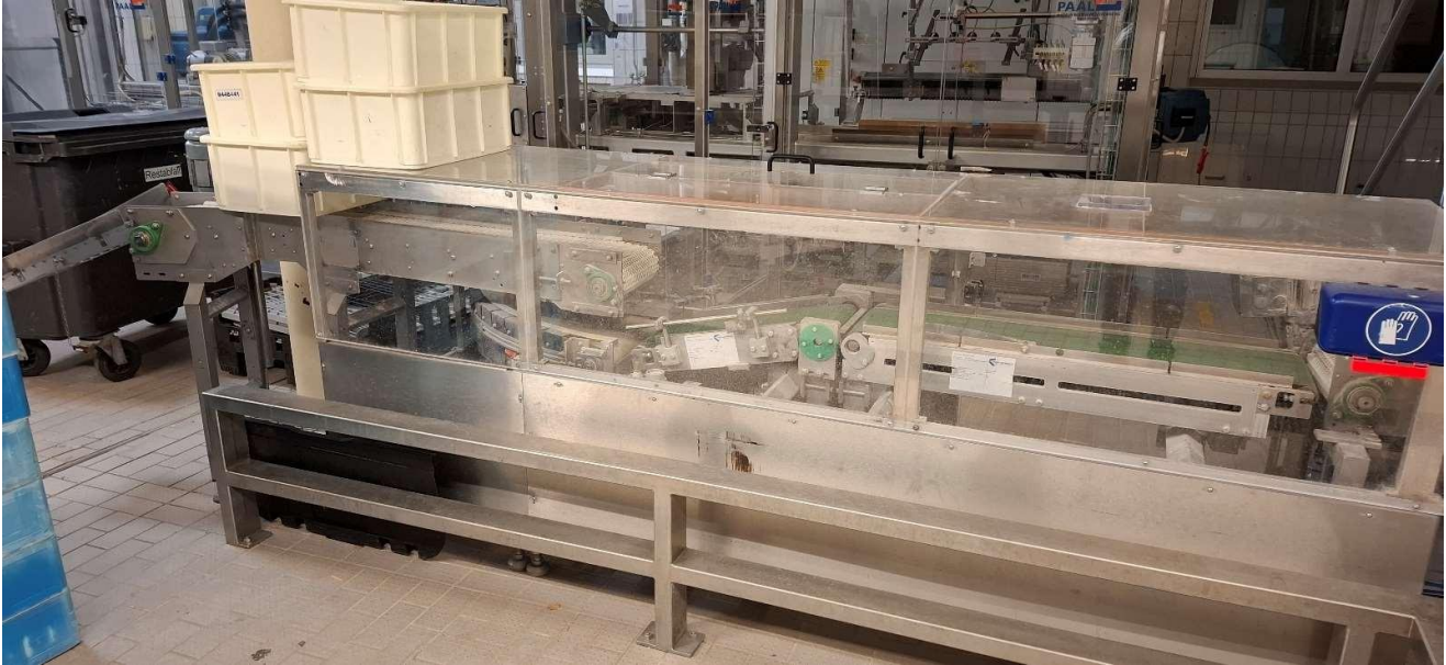
35. Discharge conveyor belt
