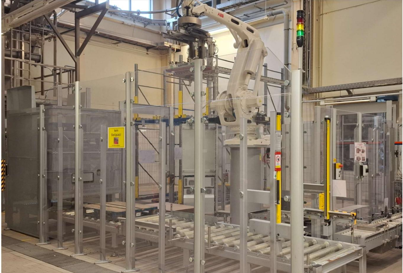
37. Palletizing system Transnovaruf
