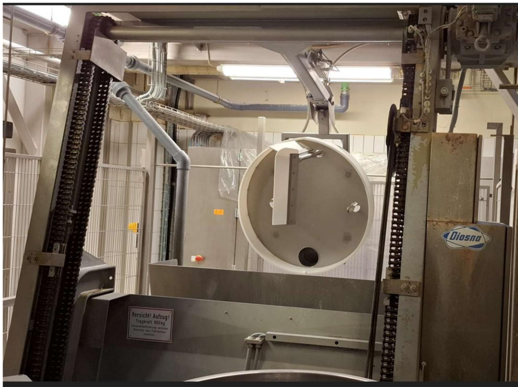
10. cleaning station for kneading bowls
