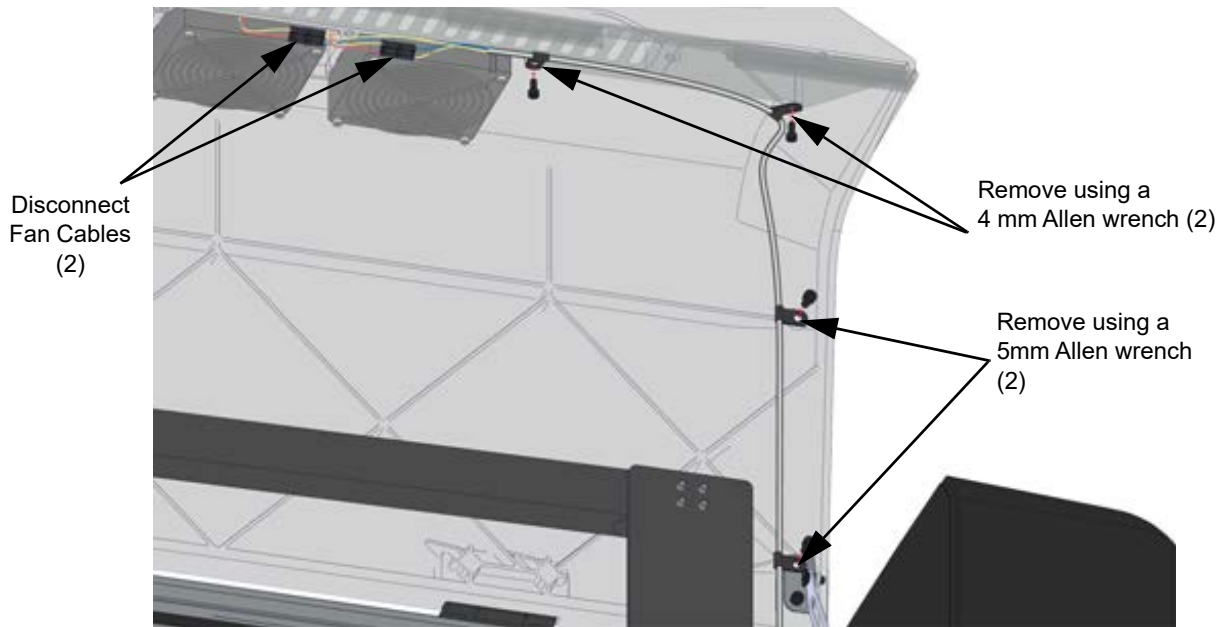
Figure 11: Disconnect Fan Wiring & P-Clamps
