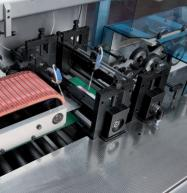
Industry proven Insert feeders eaturing suction cups, single gripper and rotary drum. Hopper height allows easy loading with high insert stack. Minimum thickness: sheet 70gr/sqm; Maximum thickness: 8 mm.
