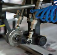
Perforator Longitudinal perforator to add a perf line for easy envelope opening
