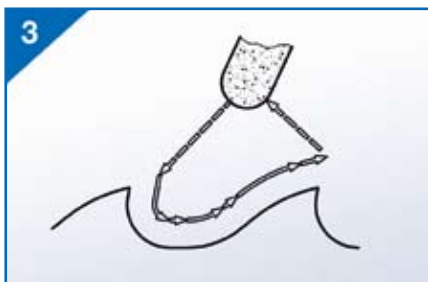
Fig. 1 – Movement of the grinding head on Bi-Metal band saw
