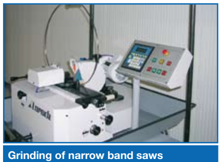
Fig. 1 – Movement of the grinding head on Bi-Metal band saw
