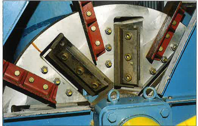
The knives are easily changed by opening the chipper hood.
