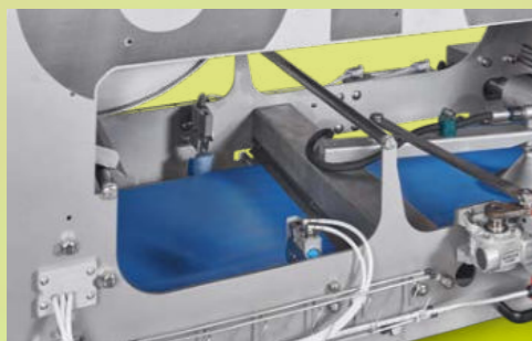
Fully automatic control of belt track
