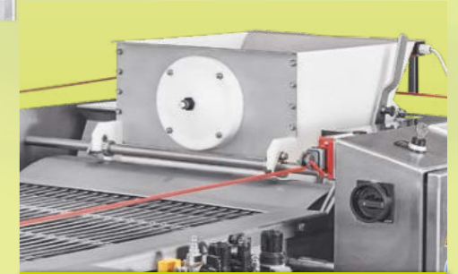
Sensor to control upstream voran® machines as washing machine or mash pump
