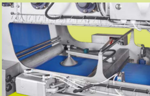
High pressure belt cleaning interval-controlled adjustable on the display
