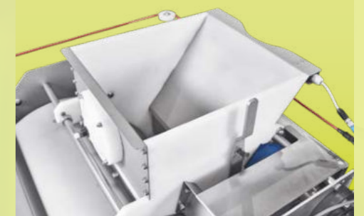
Product-specific adjustable dosing (film thickness)
