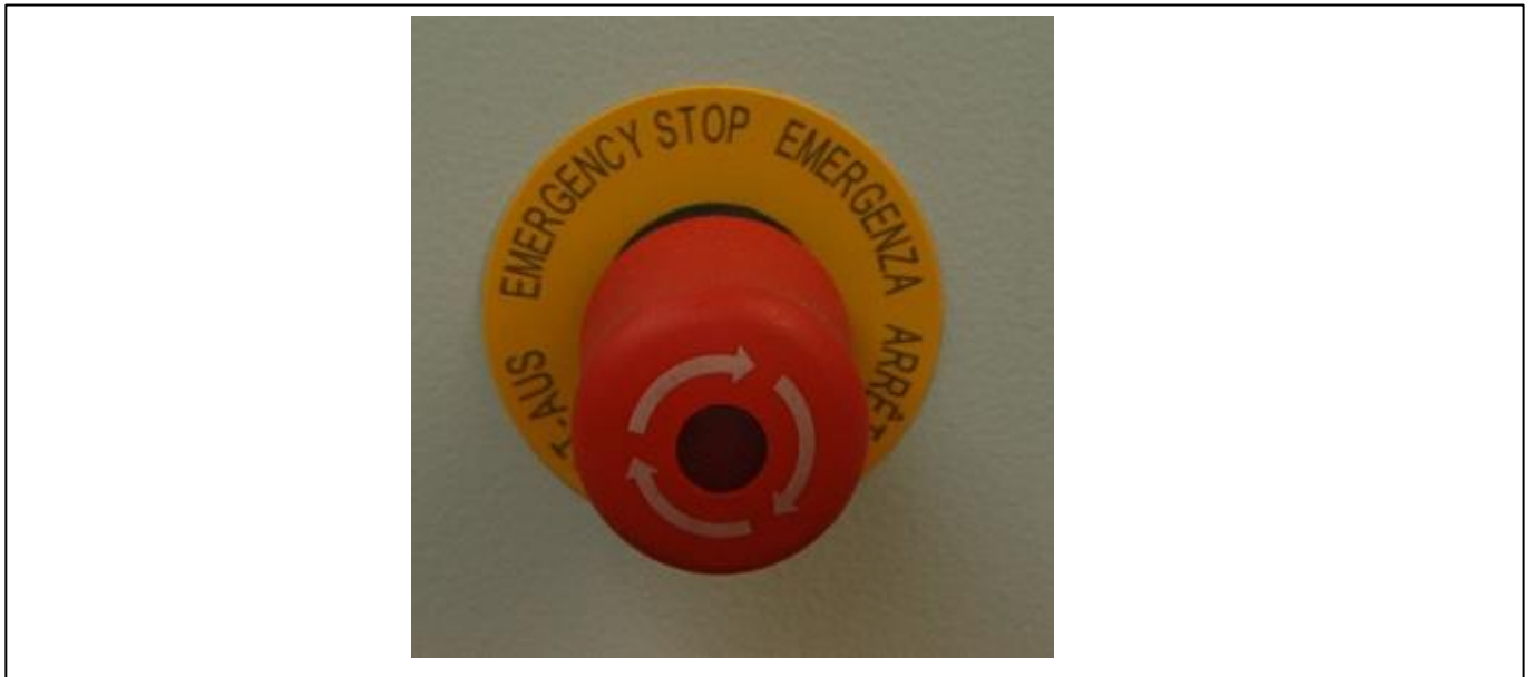
Drawing 3 Safety button - lock
