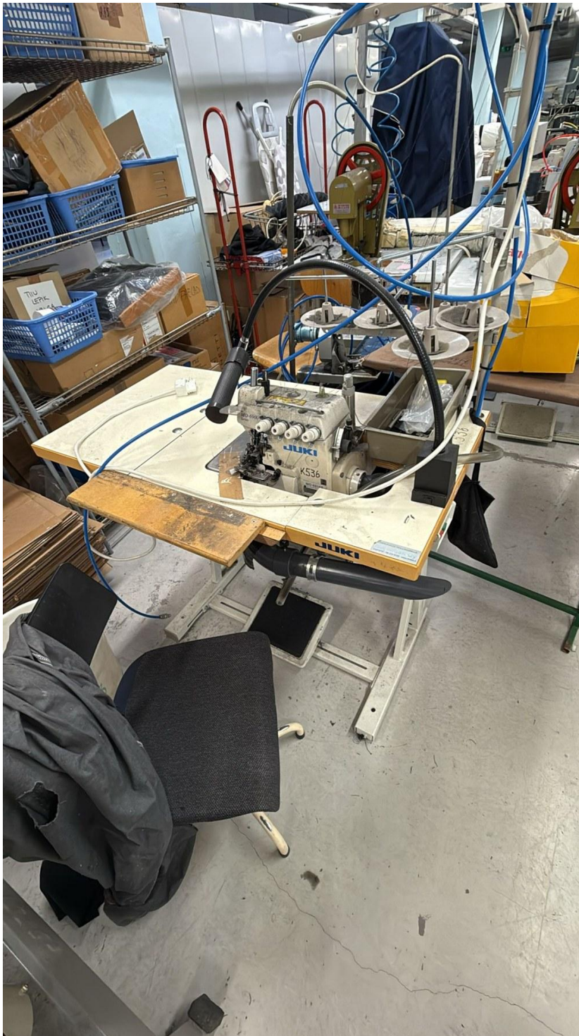
JUKI MO-6916-12 Industrial Safety Stitch Machine (2009) [132 A - K 536]
