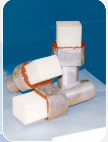
Stone supports for grinding operations. Stones with different grades according to the required surface finish quality. The stones are automatically dressed during the machining process.
