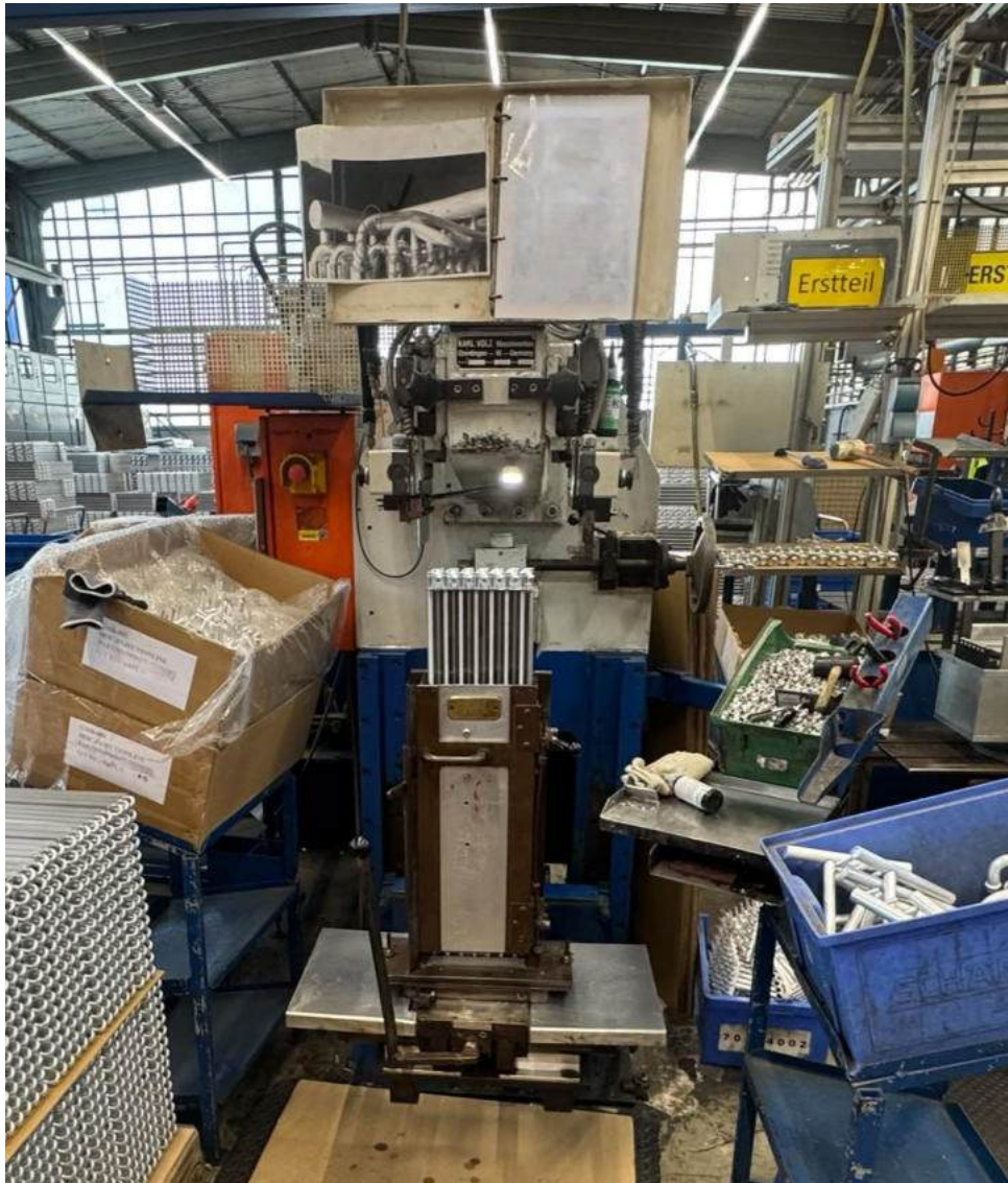
Lokring and Valve Assembly KARL VOLZ EPV 2 - 1983
