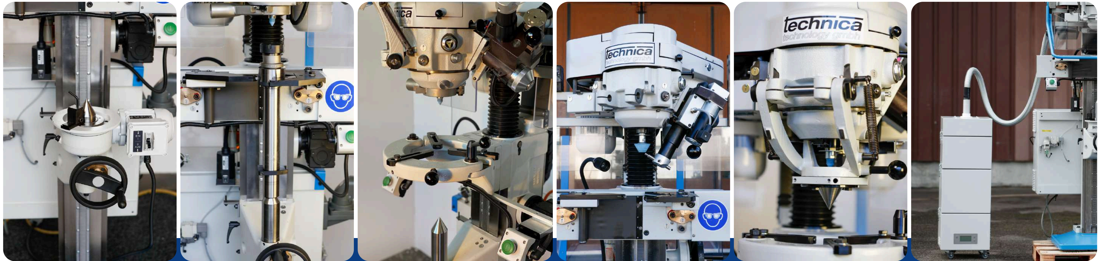
workpiece drive , collet type workpiece holder, three-point steady, dressing device, off-center point, dust extraction
