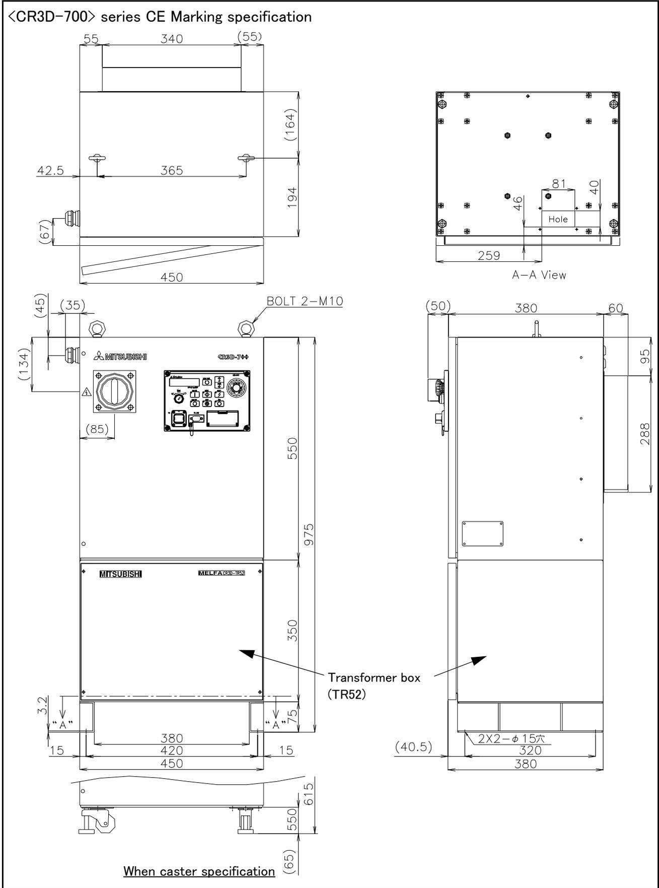
Fig.3-12 : Outside dimensions of controller(CR3D-700 CE Marking)
