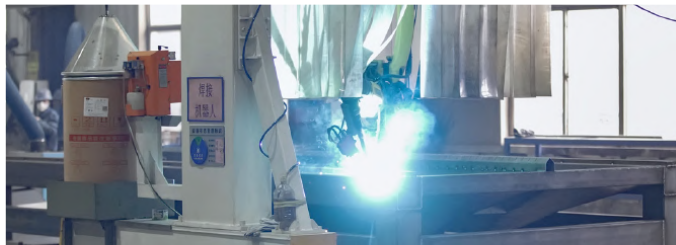
Automatic robot-assisted welding
