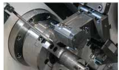
Chuck Air Blow (Upper Chuck)
