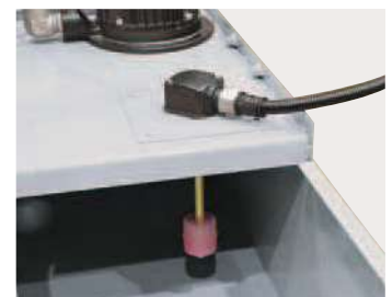
Coolant float switch
