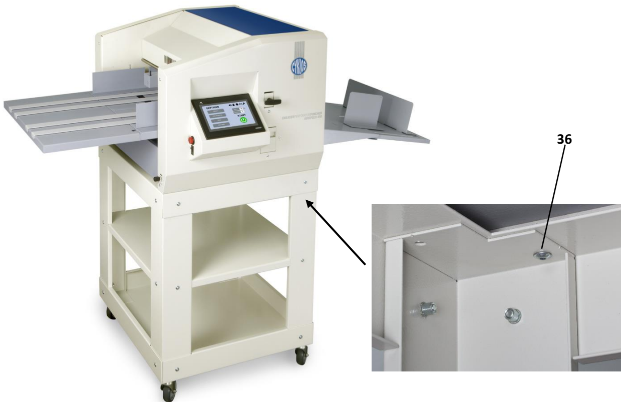
Fig. 6: Machine installation on the table
