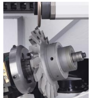
Eroding of a finishing tool.
