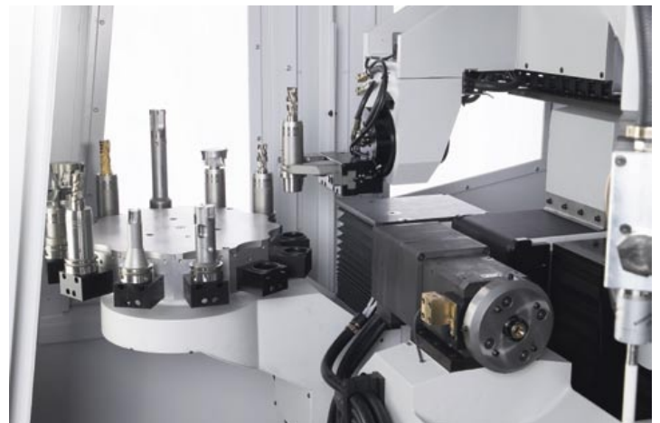
Disc erosion machine with magazine.
