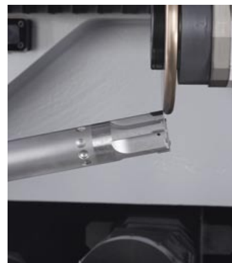
Eroding of a reamer.
