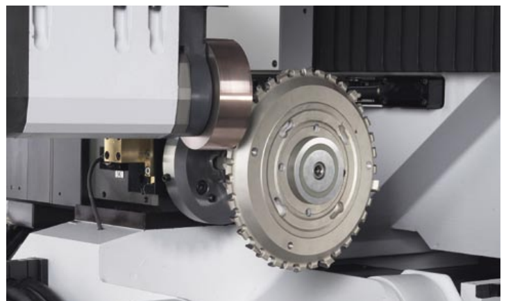
E1-axis in a swivelled position: eroding of a left-hand milling cutter.
