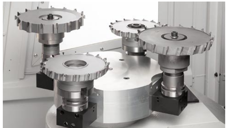
Magazine with four slots of large work pieces such as milling cutters (this magazine can also be designed as a double magazine with eight slots).
