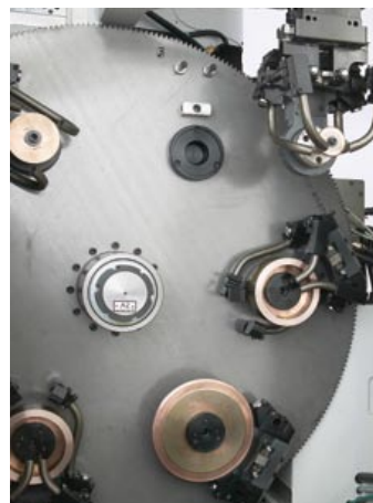
Tool magazine with six slots for eroding and grinding wheels.
