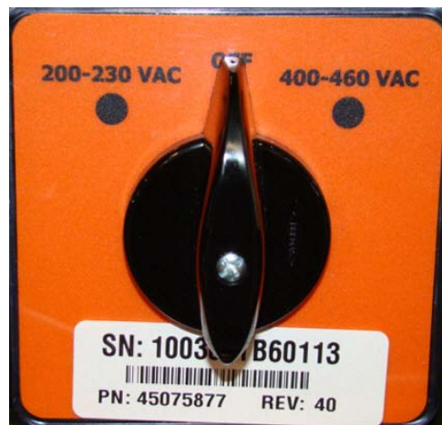
Figure 1-3: Main AC input voltage switch
