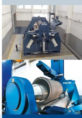
The 4HEL machines are well known for their reliability thanks to their over dimensioned structure and the centralised lubrication system. The Linear Guide Design (RGS) increases their bending precision by minimising the distance between the bending points.
