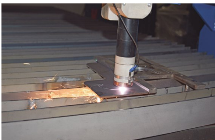
Workpiece weight is supported by catch grid. After their useful life, they can easily be reproduced
