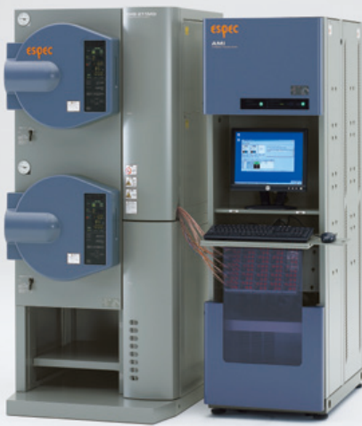
Example of the Highly accelerated stress test system with the Ion migration evaluation system
