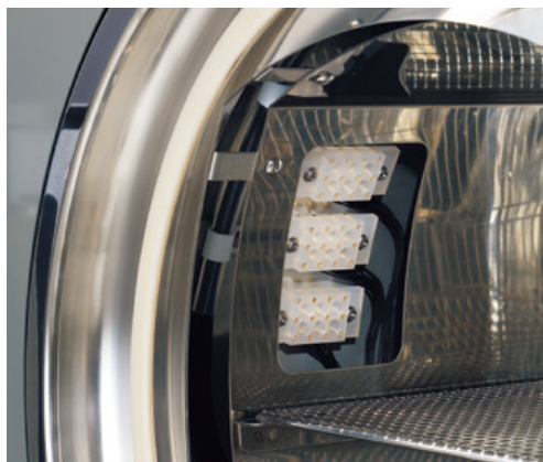
Signal terminals inside chamber
