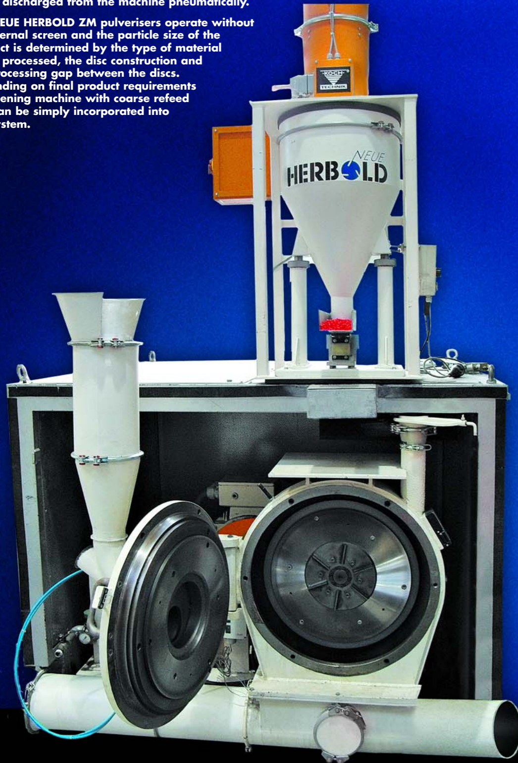
ZM 500 with sound insulation cabinet
