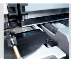
As with the mill, the spine preparation tools have reversing blades, eliminating the need for grinding or alignment. The Fibre Rougher ensures that the fibres are exposed in an optimal manner even for low-fibre paper for maximum page pull values. For a short changeover to produce thread-sewn book blocks, the stations are lowered quickly and automatically.
