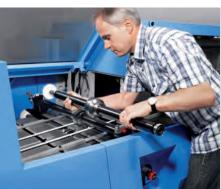
The scoring tools can be used flexibly, as they can be adapted to all types of covers. The slot width can be adjusted easily from the outside.
