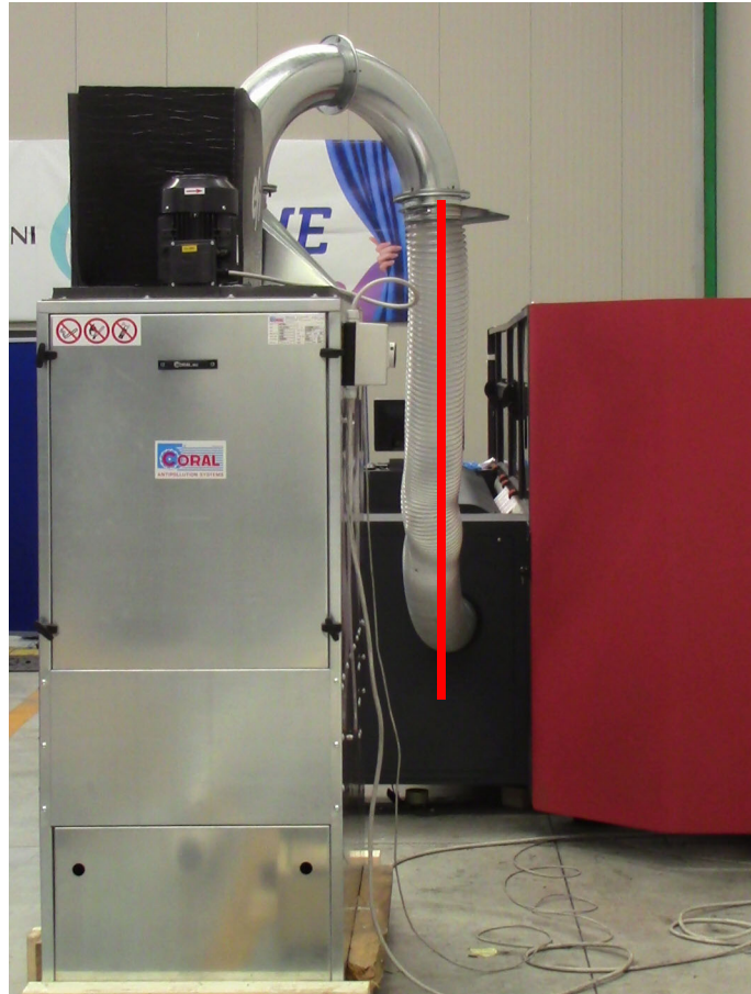
Figure 1-3: Exhaust Extraction Unit - Align Printer OUT port with Extraction unit IN port (red line)
