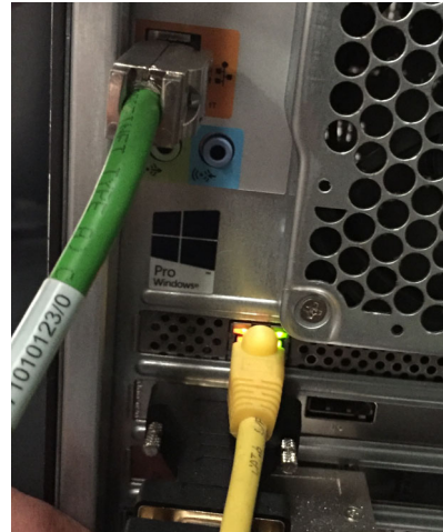
Figure 1-27: Green - Profinet cable to VIPA Service (top left) and Yellow - Internet connection, (bottom right)
