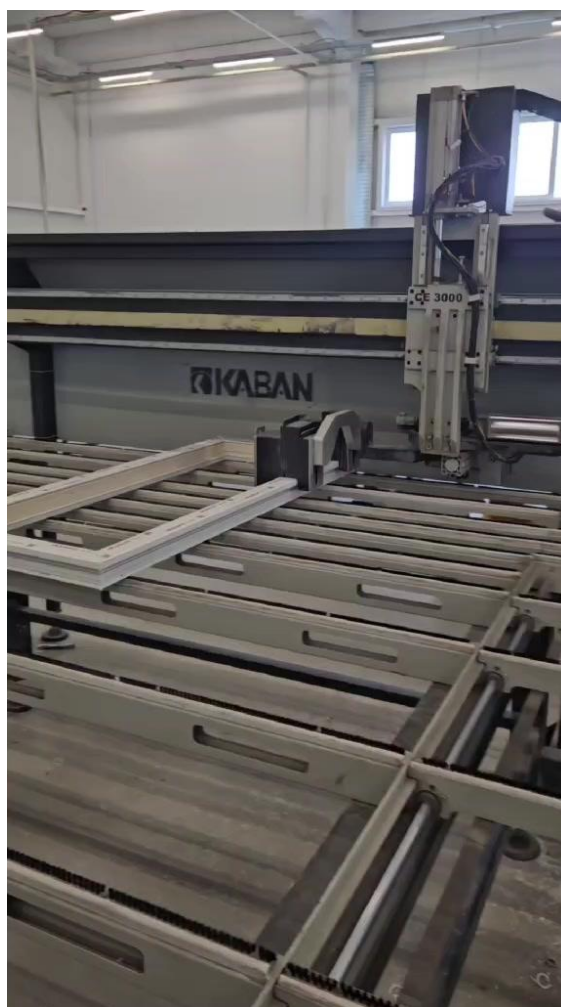
4-head PVC welding machine — simultaneously welds all four corners of the frame at 90°.
