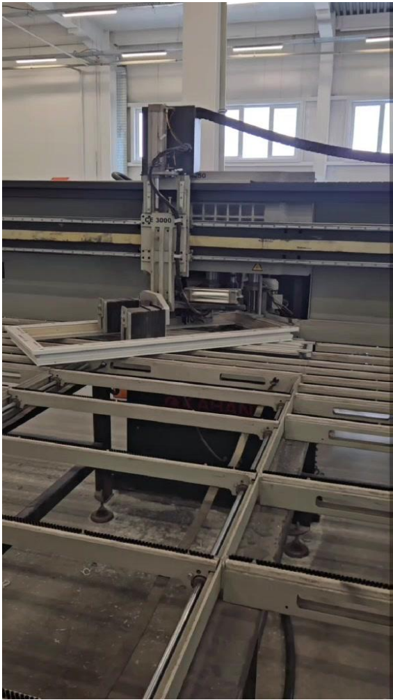
4-axis CNC corner cleaning machine with 4 servomotors — automatic cleaning of welded PVC frame corners.
