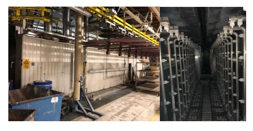
• Washing line is designed to be continuous, conveyor speed 0,7-3 m/min.
