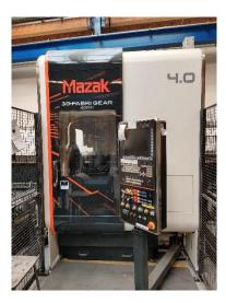
6 axis makes cutting at any angle possible for welding preparations or high accuracy assemblies.
