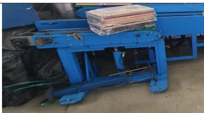
Additional conveyor to the storage table - 100 x 70 x 85 cm.
