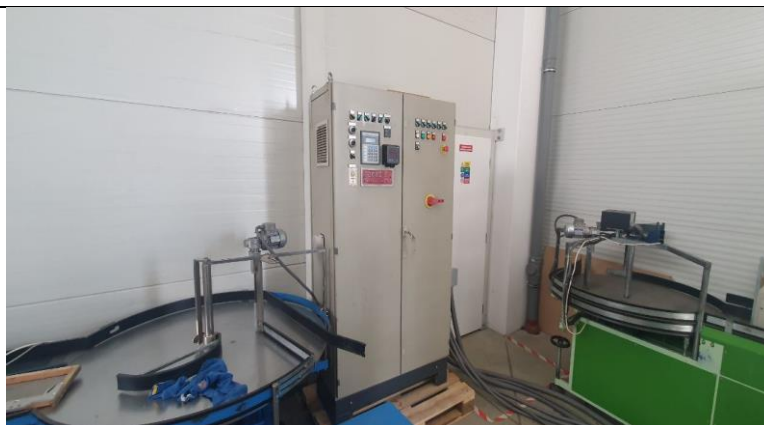
Accumulation table (green) - 400 x 140 (wide part) and 75 cm (ribbon) x 150 cm;
