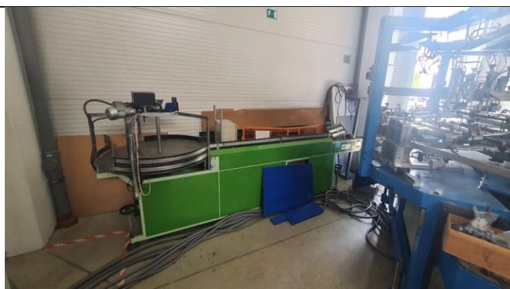
Accumulation table (blue) - 400 x 150 (wide part) and 75 cm (ribbon) x 150 cm;
