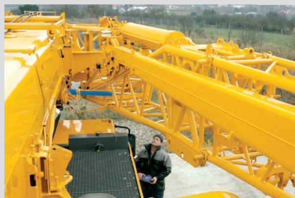
Hydraulic assembly support for attaching the swing-away jib by BTT
