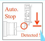
Auto Stop of manual hand feed op. when touching a workpiece.
