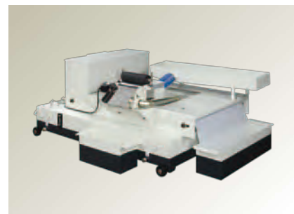
COOLANT SYSTEM WITH AUTO. PAPER FEEDING DEVICE AND MAGNETIC SEPARATOR (WITH 1 ROLL OF PAPER) B17-0302X Volume : 120L Paper feeding motor : 25W Pump : 1/8HP Coolant Capacity : 20L/min. Space :1,450 x 620mm ( 57" x 24 3/8" ) Height : 760mm (30" )
