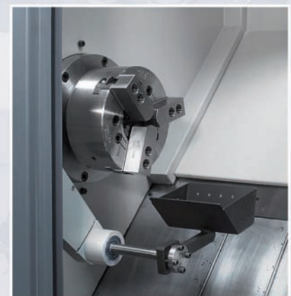
The retractable part catcher integrated with the front door outlet
