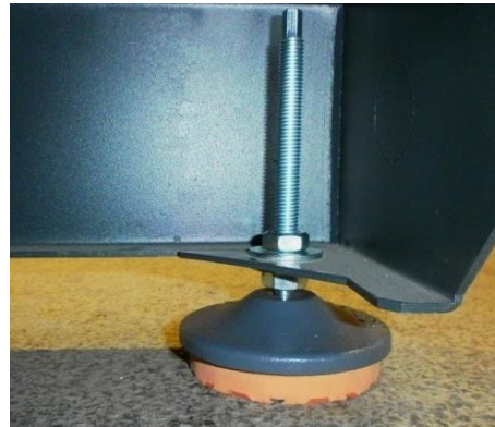
Figure 7: Machine base (foot) - mounting on the baseplate
