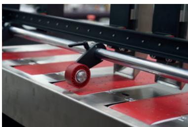
All cardboard feeding is controlled by crush weels, controlling thickness and avoiding material vibrations.
