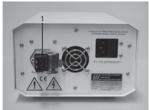
Fig. 26 Rear side of the ebq 100 supply unit
