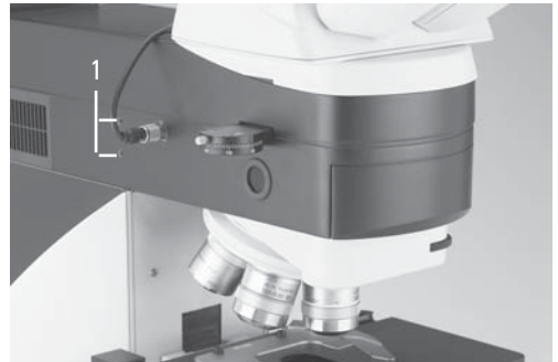
Fig. 48b Adjusting the aperture diaphragm in the incident light axis
