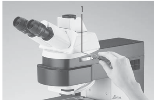
Fig. 12 Fastening the tube
