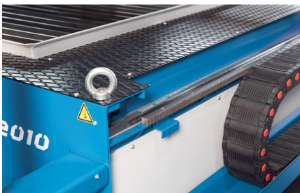
Low-wear and low-maintenance helical gears are designed for continuous operation
