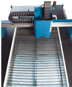
The machine is equipped with the option with 'Art. no. 253403 Water table for plasma cutting'
