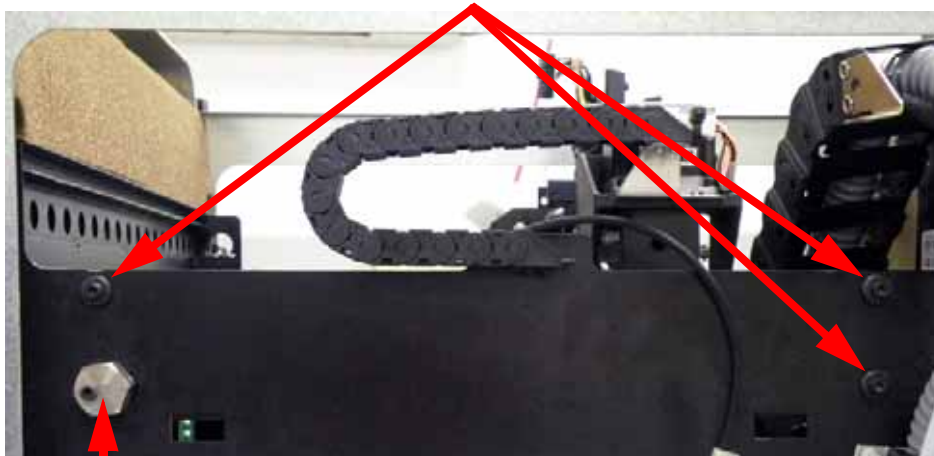
Figure 4-246: Right side cam and mounting screw locations
