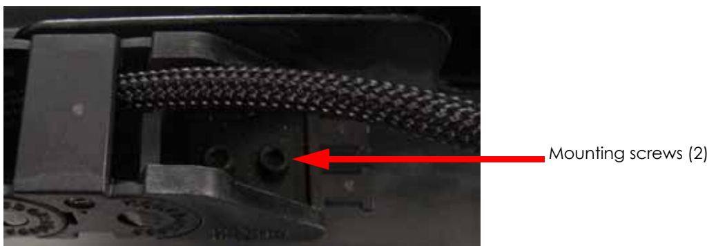
Figure 4-203: X motor energy chain lower mounting screw locations
