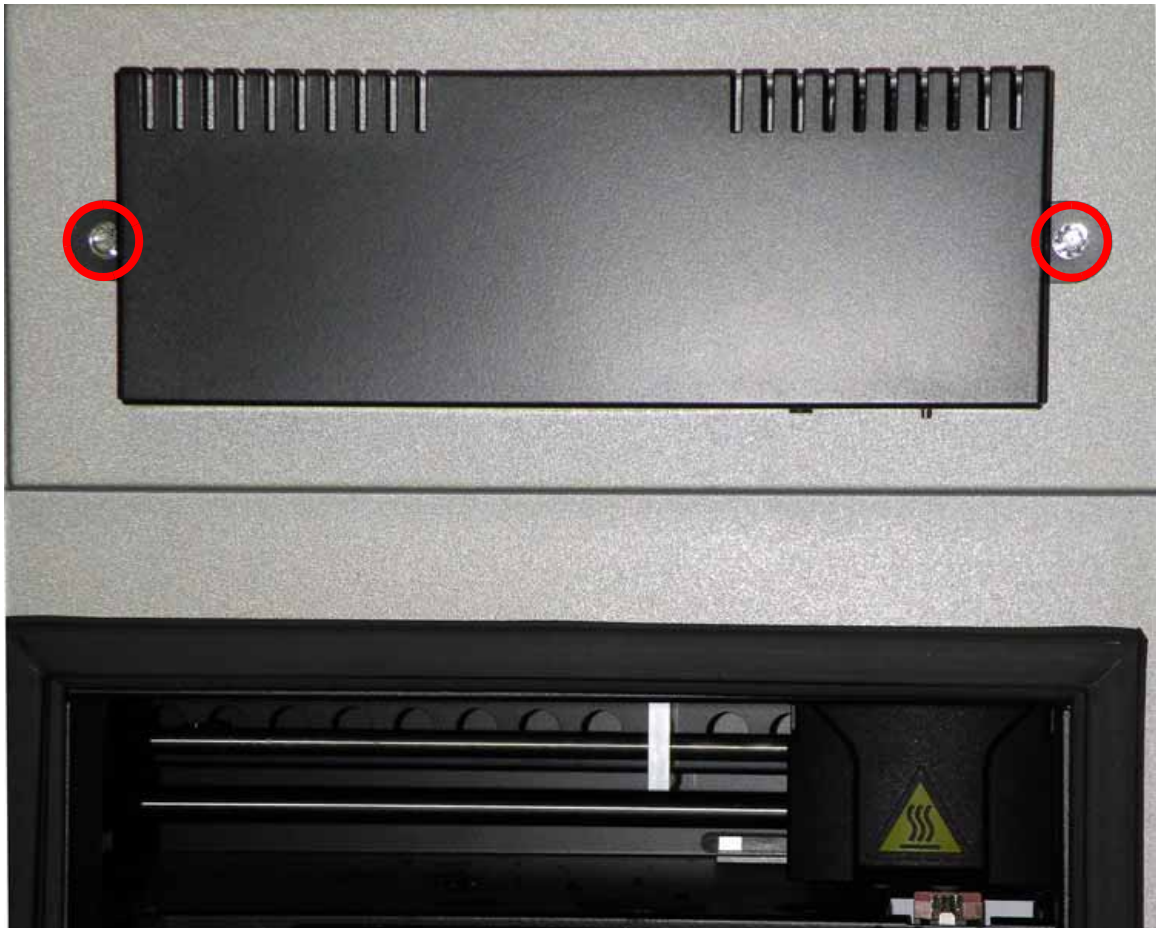
Figure 4-21: Door solenoid/sensor cover location
