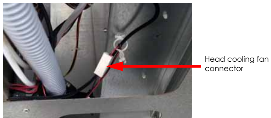
Figure 4-219: Head cooling fan connector location
