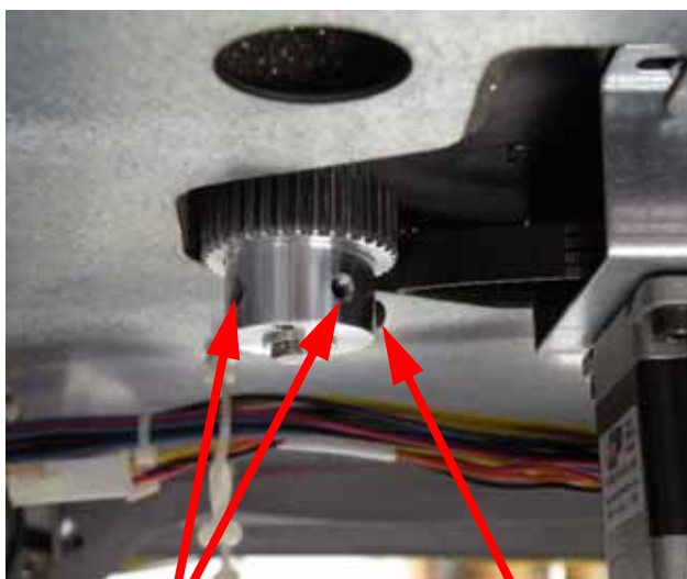
Figure 4-336: Lead screw pulley set screw locations
