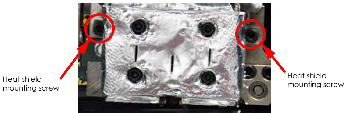
Figure 5-365: Heat shield mounting screw locations
