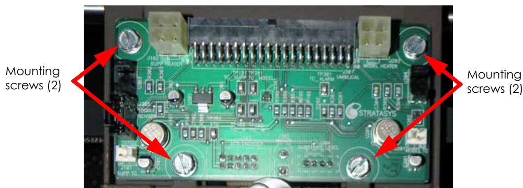
Figure 4-182: Head board mounting screw locations
