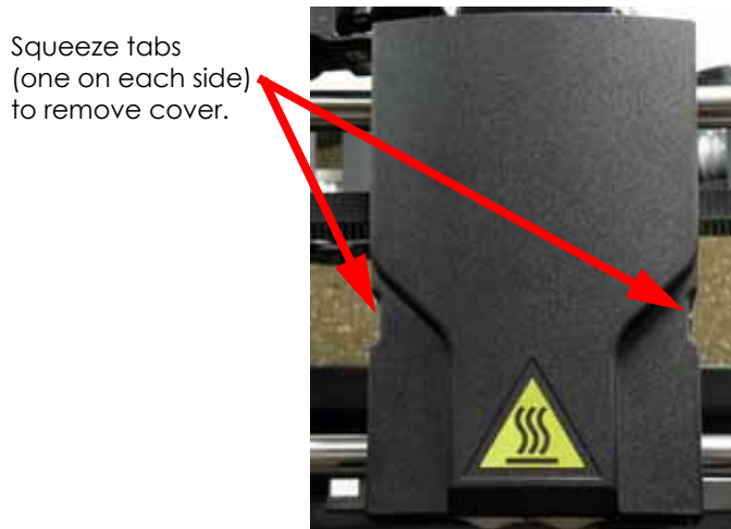
Figure 5-362: Removing the head cover
