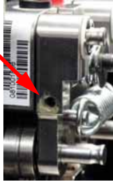
Figure 4-170: Idler Wheel Adjustment - Left Side
