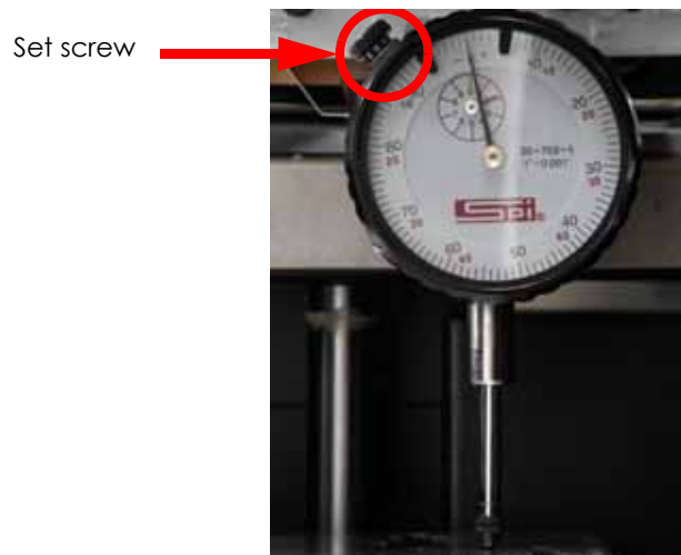
Figure 4-303: Zero the dial indicator
