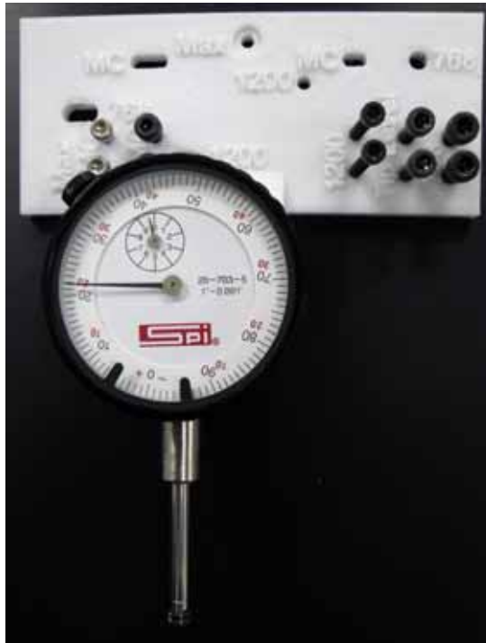
Figure 4-300: Dial indicator installation
