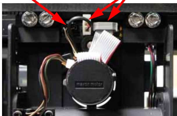
Figure 4-182: Head board mounting screw locations
