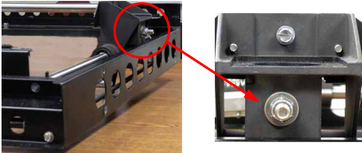
Figure 4-250: X drive belt tension nut location
