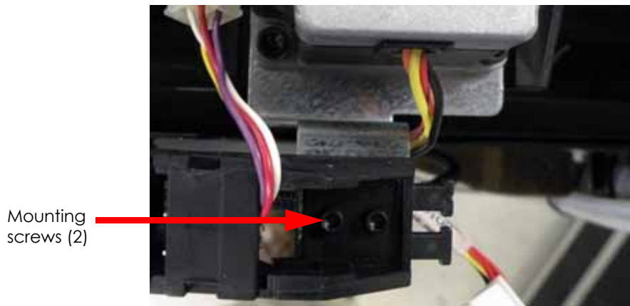
Figure 4-243: X motor energy chain mounting screw locations
