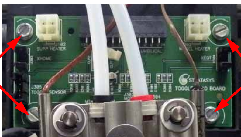
Figure 4-185: Head board mounting screw locations
