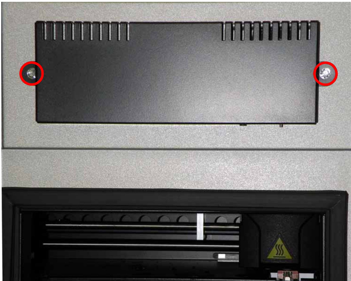
Figure 4-24: Door solenoid/sensor cover location
