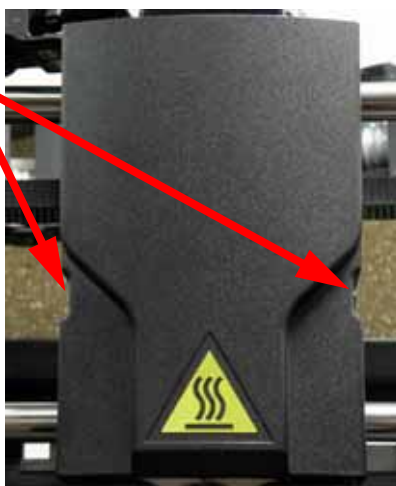
Figure 4-206: Removing the head cover
