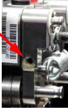
Figure 5-375: Idler Wheel Adjustment - Left Side
