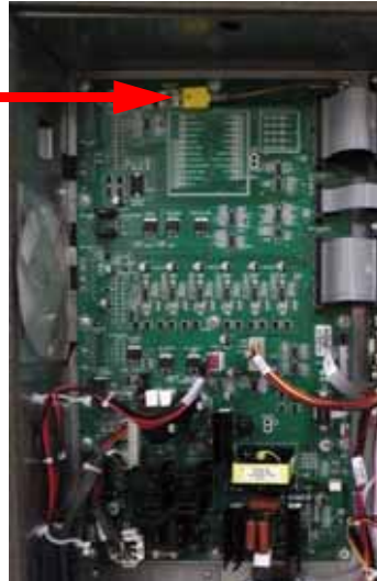
Figure 4-310: Chamber thermocouple connector location
