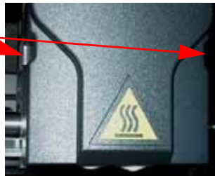
Figure 5-413: Removing the Head Cover
