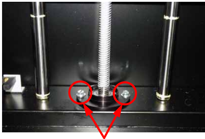
Figure 4-338: Lower lead screw bearing and retainer plate location
