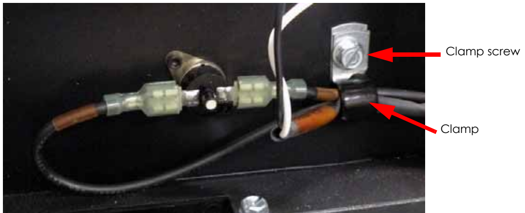
Figure 4-306: Cable clamp mounting screw location
