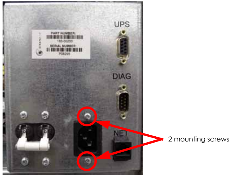
Figure 4-78: AC input mounting screw locations
