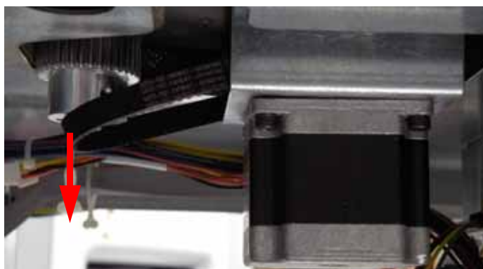
Figure 4-335: Z drive belt removal
