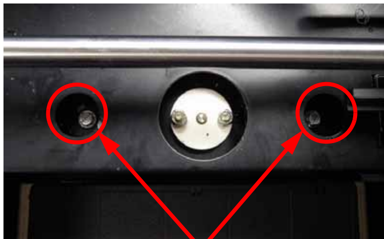
Figure 4-340: Upper guide rod screw locations
