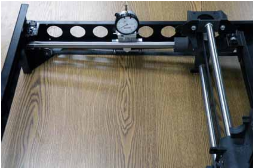
Figure 4-255: Belt tension gauge location
