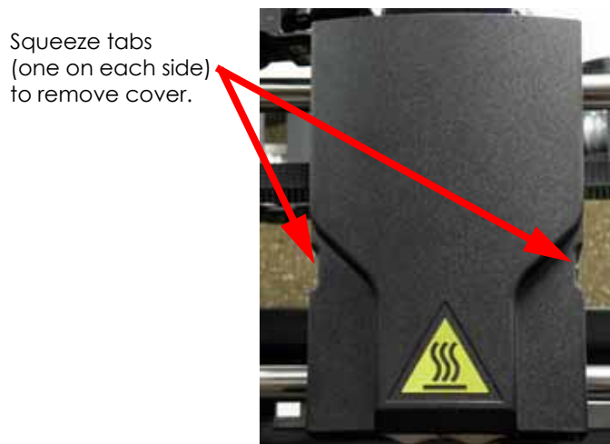
Figure 4-154: Removing the head cover
