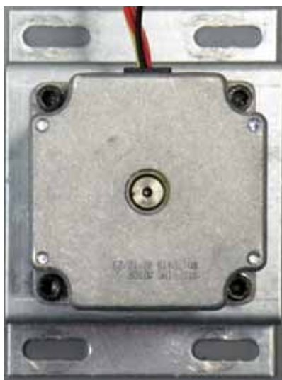
Figure 4-333: Z motor mounting screw locations
