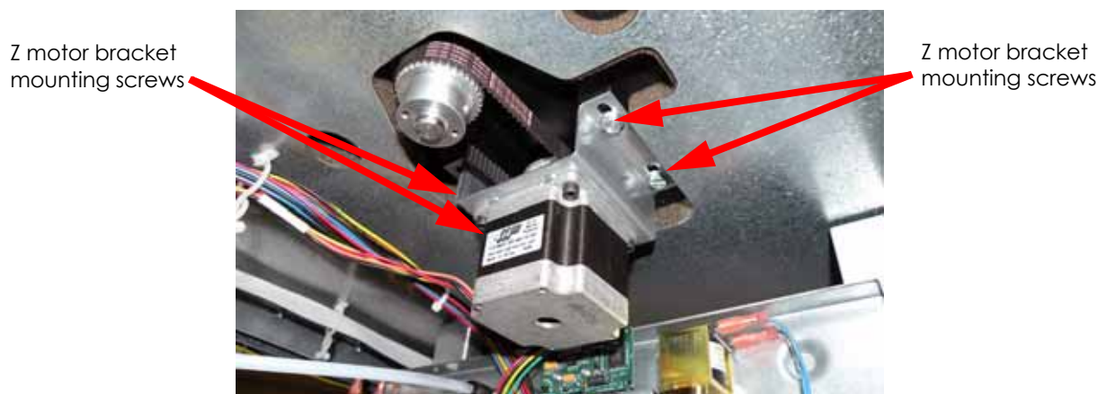
Figure 4-334: Z motor bracket and belt location
