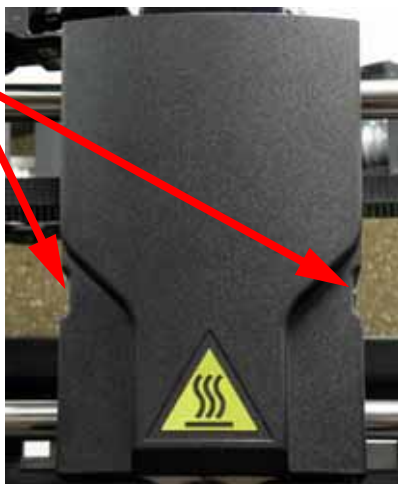
Figure 4-195: Removing the head cover
