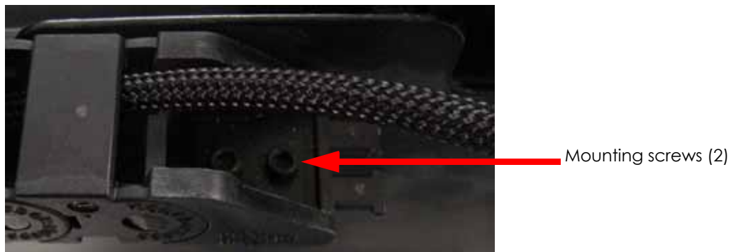
Figure 4-215: X motor energy chain lower mounting screw locations
