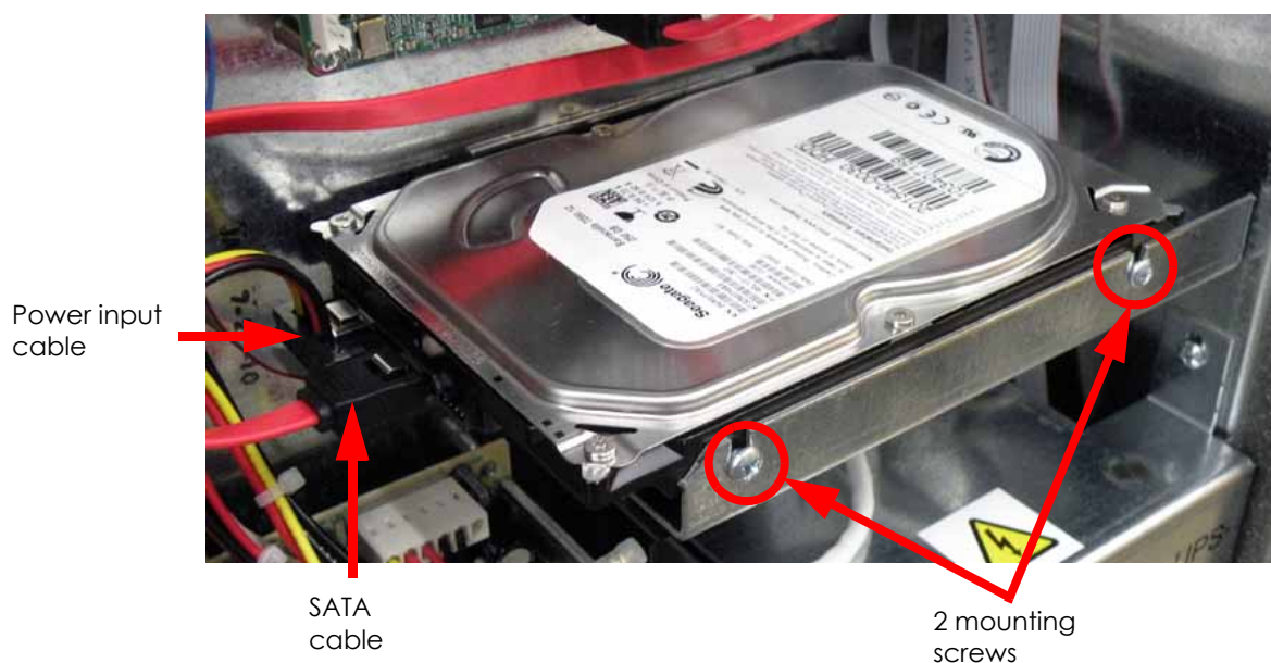
Figure 4-115: Hard drive connector locations
