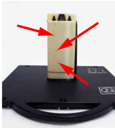
Example of embedded support
