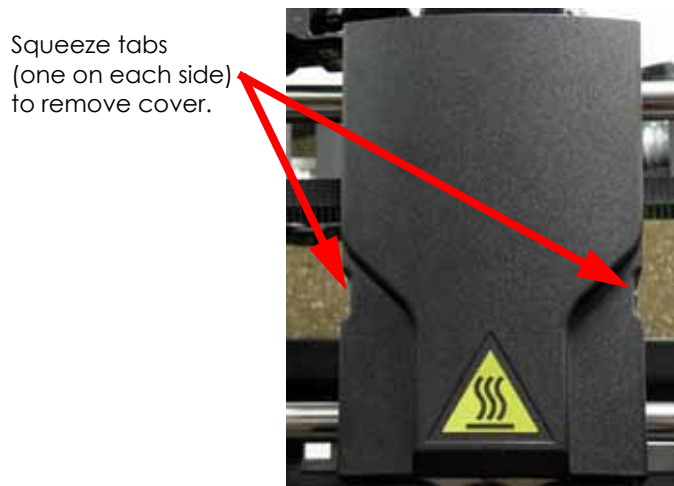
Figure 4-145: Removing the head cover
