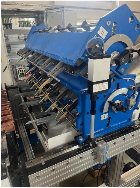
Abbildung 7: Double Cross Wire Feeder QFD34 (Layer 2. not installed in picture)
