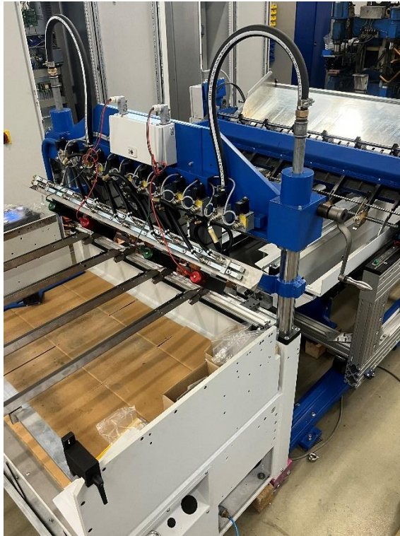
Abbildung 5: MG12 with cross wire supervision
