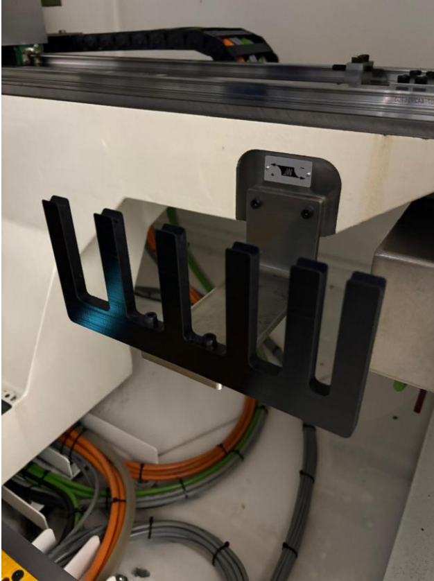
Tool rest for reversing workpiece (double ended tools).
