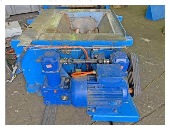
We offer you a used PET bottle crusher of the manufacturer BOREMA, type R-1200 F, year of construction 2013, for residual emptying, deaeration and pre-compaction of the fed PET bottles, from 0.3 up to 2.5 I content. The machine has a chassis and can be moved into and out of the feed chute of your baler. The machine has a throughput capacity of approx. 85,000 bottles/h, corresponding to approx. 3t/h.
