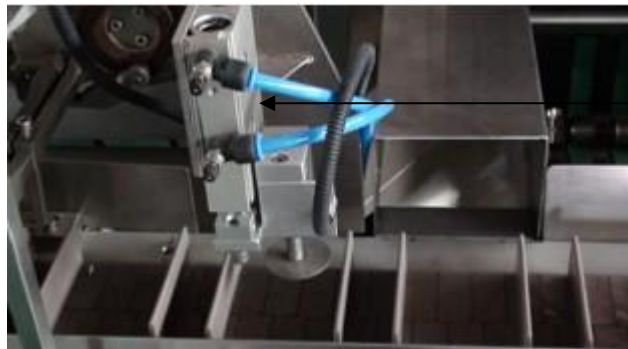
sensor detect blisters stacking height
