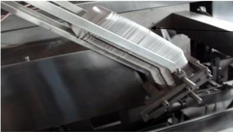
Carton magazine which can full of 400-500pcs cartons
