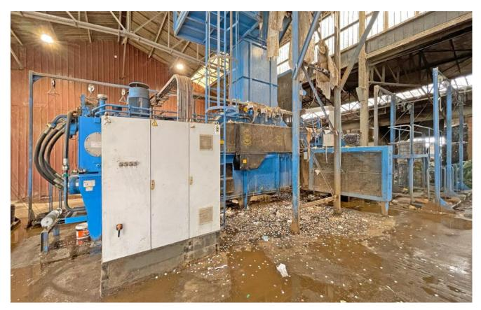
As you can see from the photos, this machine has some signs of wear that should be repaired and removed before it is used again. A basic maintenance and partial overhaul is recommended. The cylinder tube of the main hydraulic cylinder has a hairline crack and should definitely be replaced. The machine is expected to remain in single-shift operation until 03/2025 and will then be replaced by a new press with conveyor belt.
