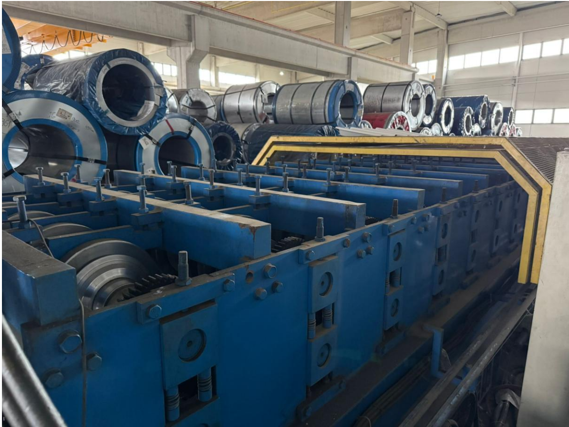
Last rolls adjustable for better optimisation of profile, making easy corrections of dimensions.
