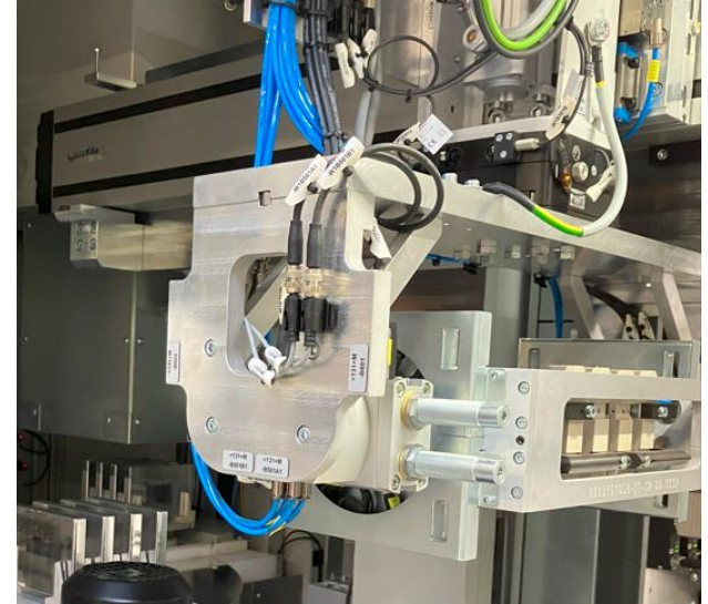
Greifer Zellhandling (gripper cell handling)
