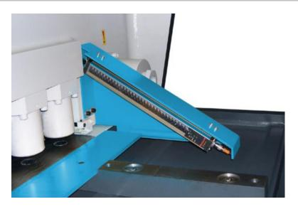
SAFETY LIGHT CURTAIN GUARDS in front of the hold downs. BALL TRANSFERS mounted in the iron table blocks, for easy feed-in of the sheets.
