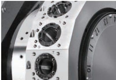
● The photo shows the bolt-tightened turret head
