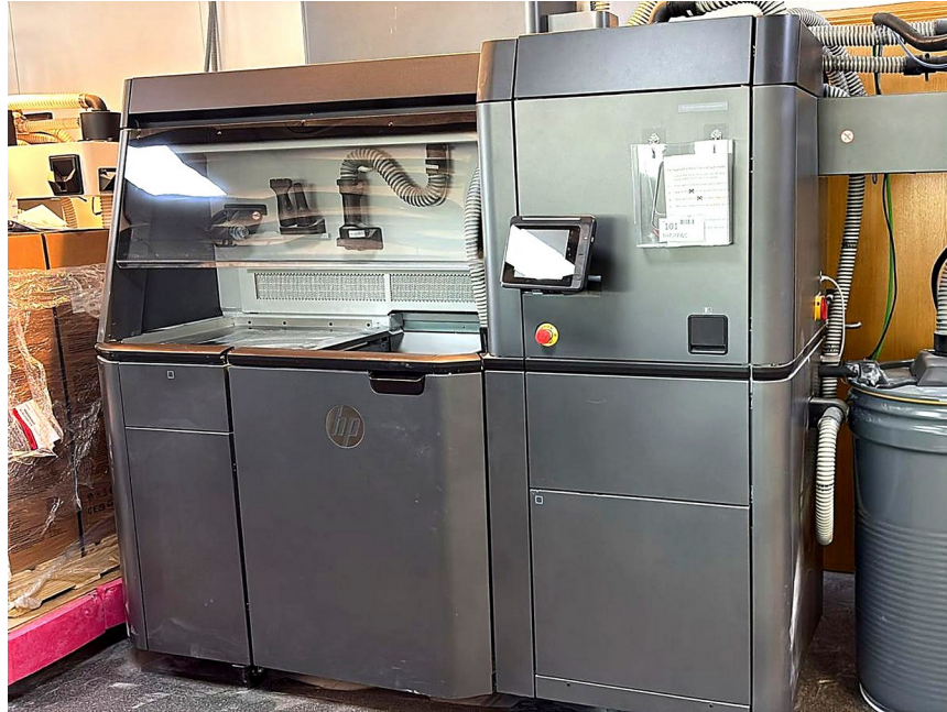
Printer, Processing Station and external powder collection, in place.
